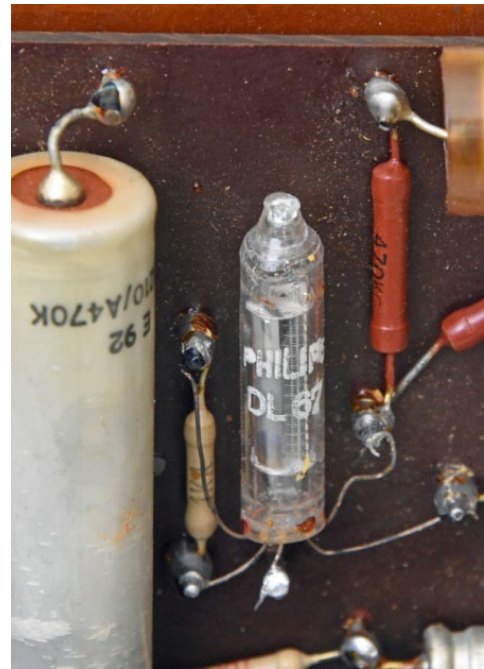
Figure 4: Detail of the circuit board containing the DL 67 pentode.
