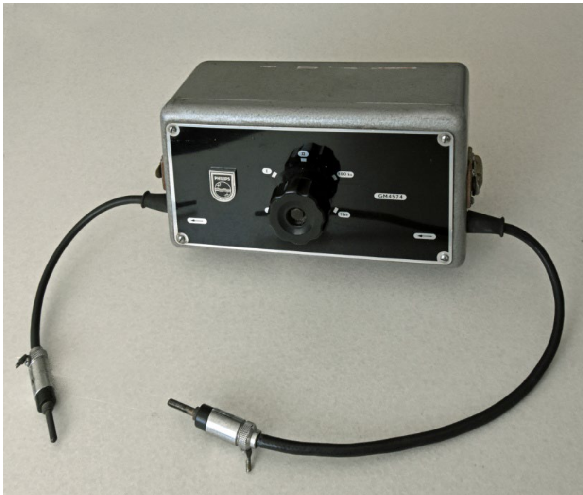
Figure 1: Amplifier GM 4574, giving an amplification of 100\times .
