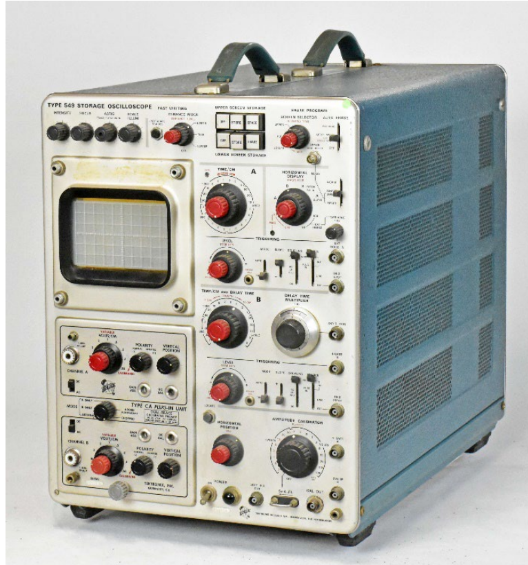
Figure 10: The Tektronix 549 storage oscilloscope; note the split screen allowing for one half of the screen as storage and the other half for conventional display as present in our collection.
