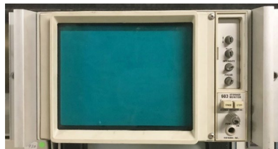
Figuur 2-80 Tektronix 603, X-Y storage monitor.
