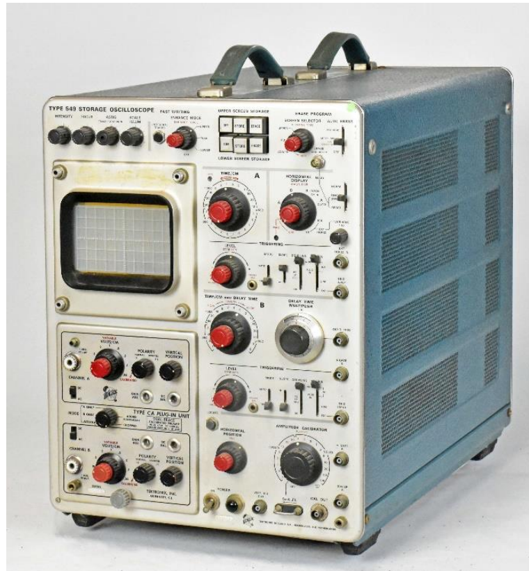
Figure 10: The Tektronix 549 storage oscilloscope; note the split screen allowing for one half of the screen as storage and the other half for conventional display as present in our collection.
