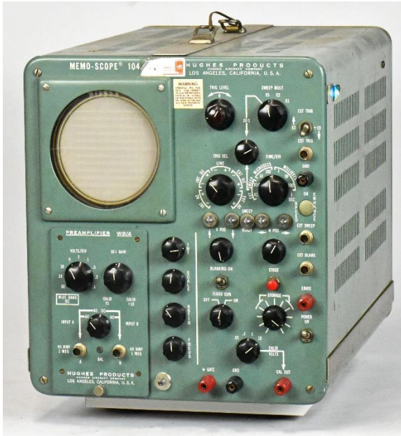
Figure 8: The Hughes 104 Memoscope (1956) as present in our collection.
