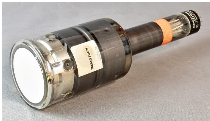
Figure 7: The Hughes Memotron type 6498 as present in our collection.
