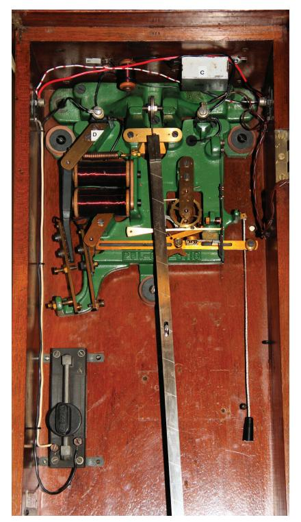
**Figure 2.** A gravity arm driven pendulum of a PUL-SYN-ETIC master clock, built by GENT of LEICESTER (1938)
