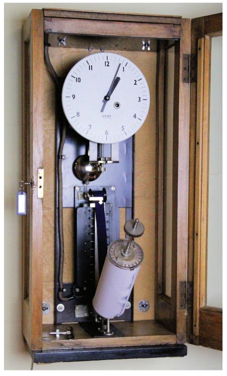
**Figure 3.** Watchman's Tell Tale Clock by GENT of LEICESTER with registration cylinder (around 1950)
