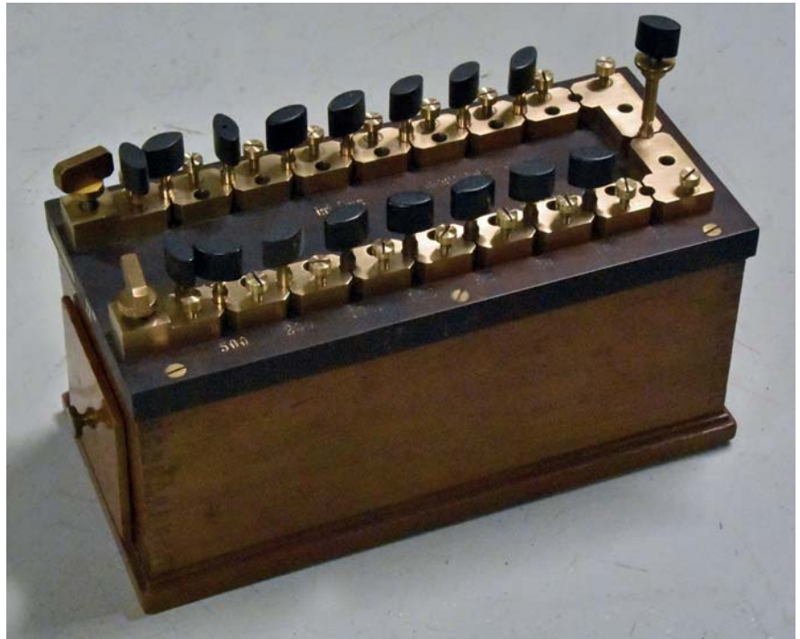
Figure 3: Resistor box with taper brass contacts, by Otto Wolff, Berlin (Photo by: Kees Pronk)
