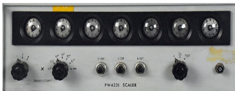
Figure 9. Philips Scaler 4231 using this special ZM 550 tube
