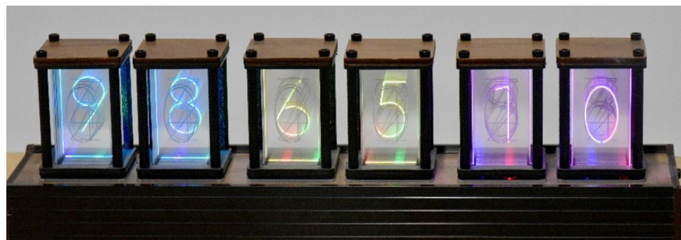
Figure 15. Modern numeric display device using LEDs
