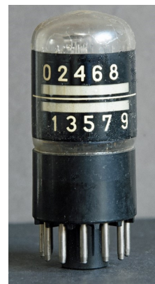
Figure 8. E1T-tube from our collection
