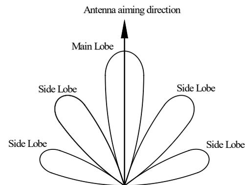
*Fig 2. Radiation Diagram of a single antenna*
