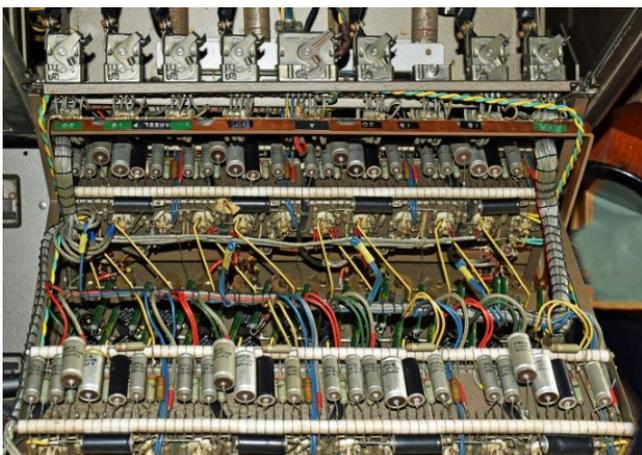
*Fig 6. Electronics for signal processing of 8 resolvers*
