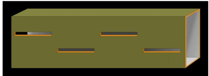
*Fig 3. Example of a slotted antenna*
